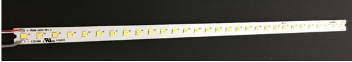
Standard LED module with 30 LED and 0.4" spacing
